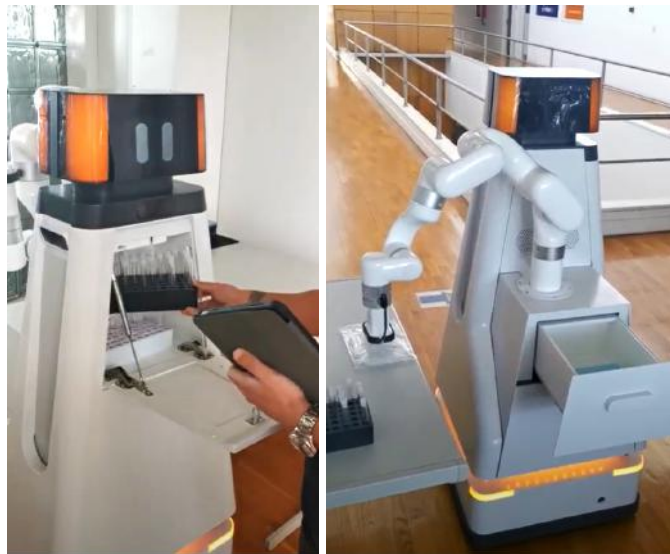
Figure 7. Behaviour of robot signalling when the “storage open”
