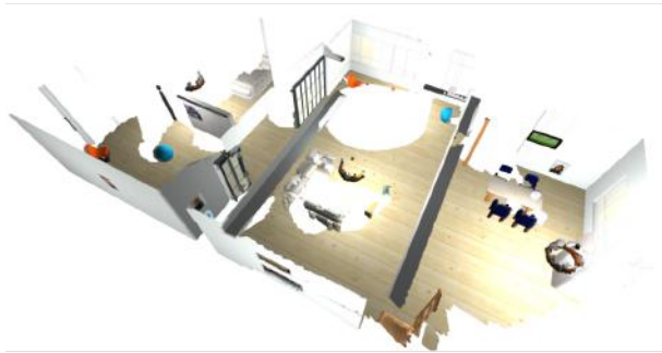
Figure 6: An example showing the output 3D map in the two stages of the autonomous model acquisition system. The object-centric model completion acquires an more complete 3D structure of the scene.
