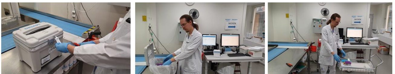
Figure 3: The box is received (left), opened (centre), and the racks are loaded on the carrier (right)
