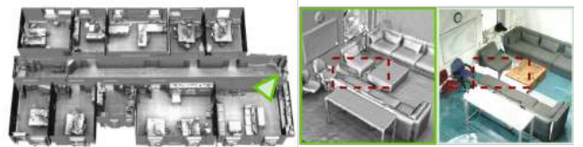
Fig. 9: Indoor mapping of the IPB office dataset. SHINE-Mapping’s reconstruction of the whole floor is shown on the left. A close-up view of the reconstructed mesh and the input point cloud of one room are shown on the right. Our approach manages to conduct reasonable scene completion in the highlighted box.
