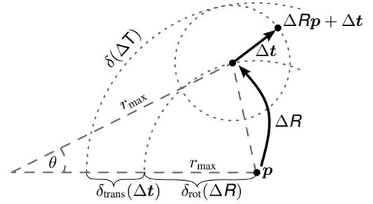
Fig. 2: Exemplary computation of the maximum point displacement  $\delta(\Delta \mathbf{T})$  caused by a rotational and translational deviation  $(\Delta \mathbf{R}, \Delta \mathbf{t})$  from the predicted motion.
