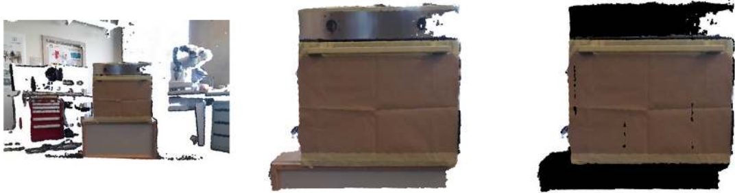
Fig. 10: Segmentation process: scene point cloud (left), object point cloud (center) and part segmentation mask (right).
