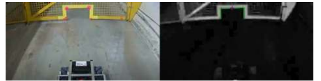
Fig. 9. Contour points (left image) used for the initialization of the segment tracker (right image).
