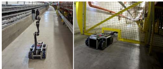
Fig. 1. The MIRA SPS Robot during inspection (left) and the MIRA Robot crossing one of the sector doors (right).
