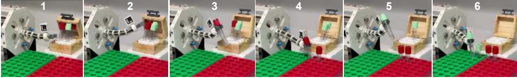
Figure 5: This set of snapshots illustrates the box opening and test tube manipulation task. In this particular task, the operator’s objective is to guide the robot in opening the lid of the box and subsequently picking and placing the tubes into the designated racks.
