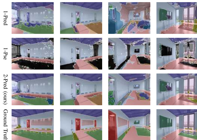
Fig. 1: Comparison of semantic segmentation performance on a recording from an indoor scene. From top to bottom: Pre-trained network predictions (1-Pred), rendered pseudo-labels leveraging multi-view consistency (1-Pse), our adapted network predictions after training on 1-Pse with a continual learning strategy (2-Pred), ground truth annotated by us. All semantic classes are color-coded. The continually-learned network produces more view-consistent predictions than the pre-trained network, as visible for instance for the desk. In the second row black indicates that no semantic class can be determined, due to the missing depth information.
